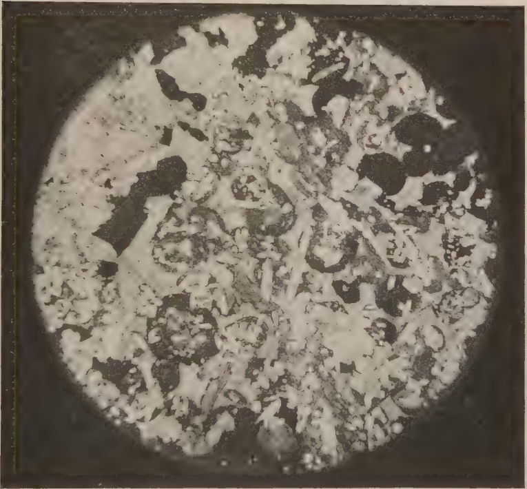
(16) Photomicrograph (x12) of section of oolitic Ste. Genéviève limestone from footwall of Mary Belle mine showing replacement of rock by quartz crystals (clear, light patches bounded by sharp edges) and zinc blende (black).
